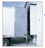
If off-center trailer contact occurs, the S-3200 moves upward and back, preventing costly damage to the wall and shelter. After the truck leaves, a gravity-biased design returns the frame to its original position.
